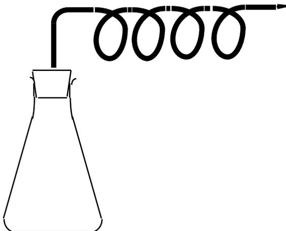
Place a Meker burner under the coil. Heat the flask on the hot plate. Once steam starts to escape the coil, heat the coil with the Meker burner. The superheated steam coming from the coil will be well over 100°C. After a minute of heating, the steam will scorch a piece of paper in the path of the steam and may cause the paper to burst into flame.
