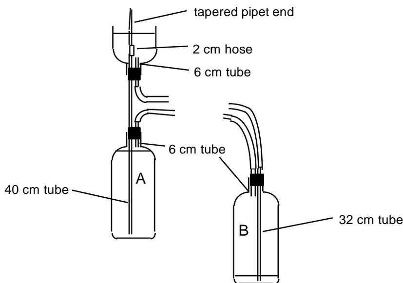
Fill bottle A with water, put about 2 cm of water in bottle B (just enough to get the water level above
